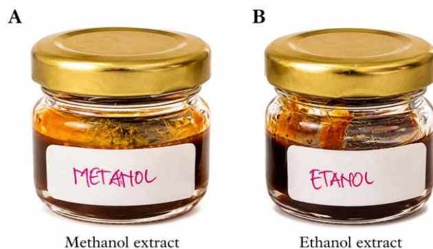
Figure 1. Results of esterification of stingless bee hive waste extract using methanol (A) and ethanol (B). The methanol and ethanol esterification products showed comparable yields, indicating that both alcohols were suitable for ester formation under the sonochemical reaction conditions.
